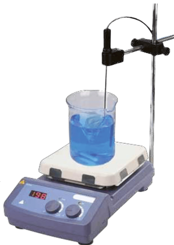
Stirrer with adjustable stand and PT 1000 probe
