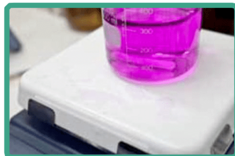
Glass ceramic hotplate with high chemical resistance
